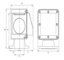
10-APH-SS-S – Fabricated Air Pipe Head 10?
