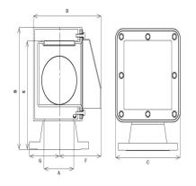
10-APH-SS-W – Fabricated Air Pipe Head 10?
