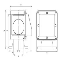
12-APH-SS-F-P-C – Fabricated Air Pipe Head 12?
