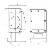
12-APH-SS-S-P-C – Fabricated Air Pipe Head 12?
