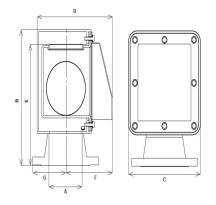
12-APH-SS-T-C – Fabricated Air Pipe Head 12?
