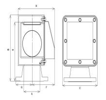
12-APH-SS-T – Fabricated Air Pipe Head 12?
