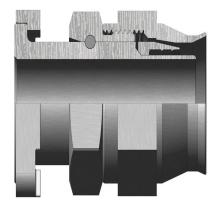
148-05204-10 – Medium Pressure TFE Flared Hose Fittings – 45° Elbow, Flared, Bent Tube
