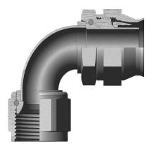
148-05208-10 – Medium Pressure TFE Flared Hose Fittings – 90° Elbow, Flared, Bent Tube
