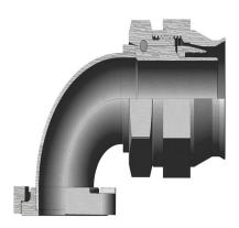
148-05210-10 – Medium Pressure TFE Flanged Hose Fittings – 90° Elbow, Flanged, Bent Tube
