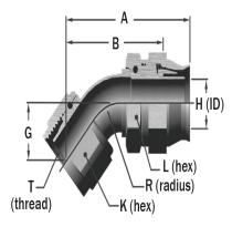
148-05219-10 – Medium Pressure TFE Flareless Hose Fittings – 45° Elbow, Flareless, Bent Tube
