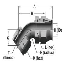
148-05219-16 – Medium Pressure TFE Flareless Hose Fittings – 45° Elbow, Flareless, Bent Tube
