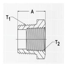
8645-12-8-CUNI – 8645 Series Reducer-Male External NPTF x Female Internal NPTF Adapters
