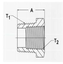
8645-16-12-CUNI – 8645 Series Reducer-Male External NPTF x Female Internal NPTF Adapters
