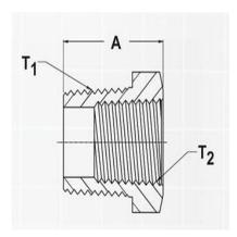
8645-16-8-CUNI – 8645 Series Reducer-Male External NPTF x Female Internal NPTF Adapters
