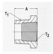
8645-4-2-CUNI – 8645 Series Reducer-Male External NPTF x Female Internal NPTF Adapters
