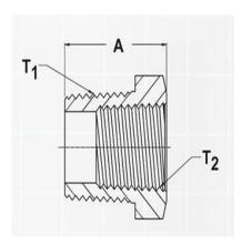
8645-6-4-CUNI – 8645 Series Reducer-Male External NPTF x Female Internal NPTF Adapters
