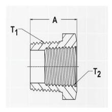
8645-8-4-CUNI – 8645 Series Reducer-Male External NPTF x Female Internal NPTF Adapters
