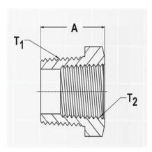
8645-8-6-CUNI – 8645 Series Reducer-Male External NPTF x Female Internal NPTF Adapters
