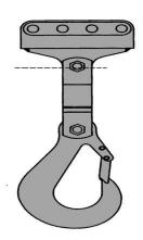
ADP/AY-CH/STROL - Cargo Hooks - Stream Trolley Assembly
