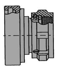
B-ADP/SW-4FS-25FHT - Adapters - Female Split Clamp to Female Hose Thread Swivel
