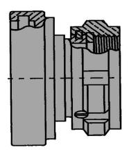
B-ADP/SW-4FS-4FHT – Adapters – Female Split Clamp to Female Hose **Thread Swivel**
