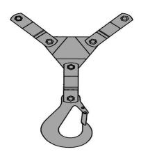
ST-HST/AY - Hooks - Hoisting Assembly (MK20 MOD O)
