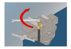
3. The insert is then threaded into the socket and hose. Leave  $^{1}/_{16}$  inch clearance so nut is free to swivel.
