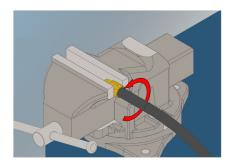
1. Screw hose into socket (left hand thread) until it bottoms. Back out hose 1/4 turn.
