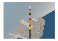
2. Slide the insert onto the mandrel. Lubricate the hose ID and the insert of the sub-assembly with lubricating oil or light grease.
