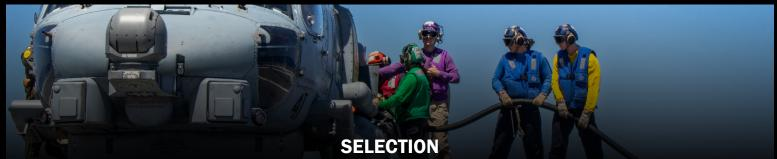
Hydrasearch offers Aircraft Ground Refueling Hose Assemblies, collapsible and non-collapsible, in 1½" and 2½" diameters per MIL-DTL-17902. Additionally, we offer Aircraft Refueling Hose Assemblies from 1" - 6" in diameter according to the specifications listed below.
